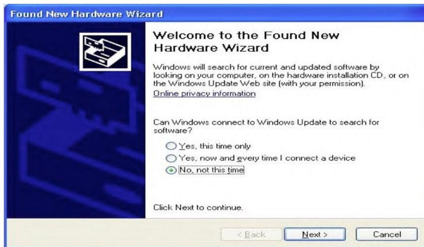
If the PC has Internet Access you may be able to set the “Yes, this time only” button and click Next for the PC to find and install the right driver. Advice may also be obtained from the FTDI website on how to obtain a suitable VCP driver for their USB chip.
