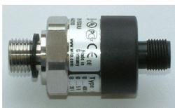
A pressure transducer is used to monitor the forward hydraulic pressure in the boom lift ram. The pressure sensor connects to the angle sensor module by a 4 way M12 cable. The forward pressure reading directly relates to the load lifted by the machine. The sensor measures up to 400 Bar.
