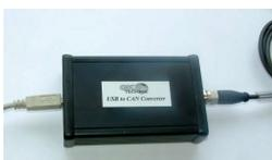
A USB to CAN Converter Interface is used to allow a PC to communicate with the Series 1-L during initial set-up and for later monitoring purposes.
