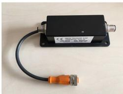
The Angle sensor should be fitted to the first excavator boom and connected to the pressure transducer that is fitted to the main lift rams. The sensor is connected to the display via a M12 OCAN bus cable. An LED on the Angle Sensor flashes green to show that it is powered and working correctly. Where possible, ensure that the green LED on the Angle Sensor is visible during operation to show the Angle Sensor is working correctly.
